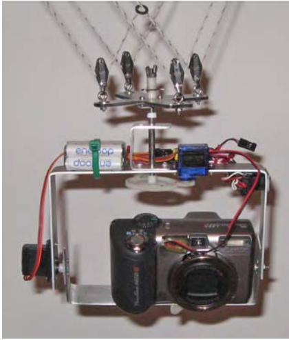
Figure 9-9. A pan/tilt rig made for a camera using two servos (image by David Mitchell)
