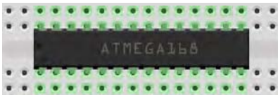
Figure 2-3. An Integrated Circuit (or chip) plugged across the gap in a breadboard
