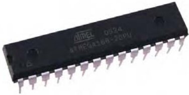
Figure 1-22. An Atmel ATmega chip, the heart of your Arduino. (image courtesy of Earthshine Electronics)
