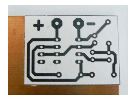
3. Drill the holes with 0.8mm or 1mm drill and cut out the board:
