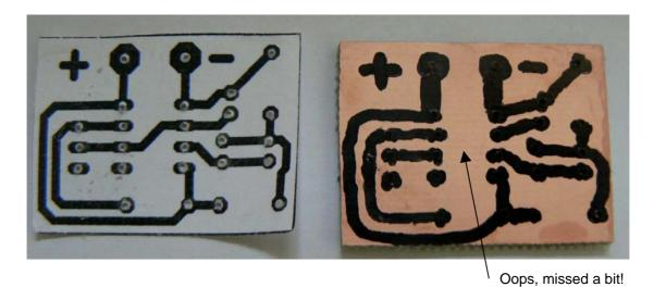
5. Etch the board and sand off the etch-resist:
