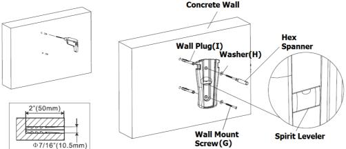
For plaster wall installation first of all find out where the wood stud is behind the wall using a stud finder. Then work out the height of the installation and ensure it is level using the spirit level. Use a pencil to mark where the mounting holes will be and use an electric drill to drill a hole that is around 4.5mm in diameter and 50mm deep. Install the wall bracket as follows.
