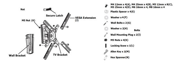
For this installation you will also require a pencil, tape measurer, electric drill, stud finder and a Philips (cross) screw driver.
