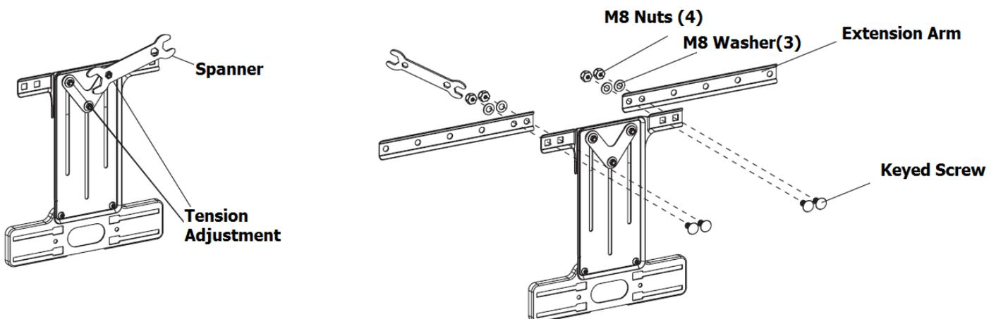
**Step 2** – Slot in the support arms and slide them to the end of each side. Insert the stopper plugs into the holes to fix the arms in place.
