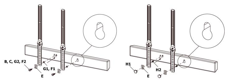
STEP 3 – Attach soundbar and bracket to a TV bracket
