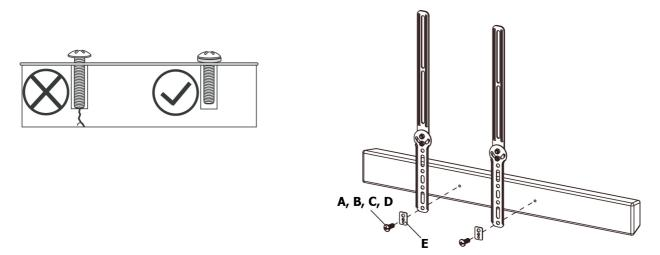
If the soundbar has keyhole inserts then install the brackets either way as pictured below.
