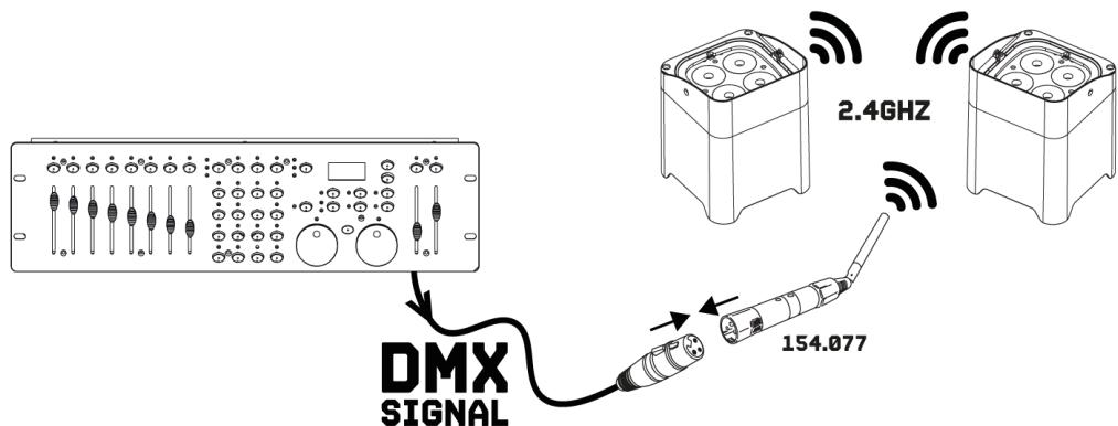
Set BBP W-DMX transmitter and receiver into operation by connecting its power unit to the power input and the mains plug to a mains outlet (100-240V~, 50/60 Hz). The status indicator shortly flashes red.
