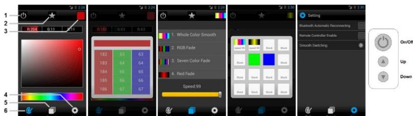
The ColorEasy3 Plus app has 3 edit screens for Static (6), Dynamic (5) and Setup (4) menus. In Static mode, a slide bar sets the hue and a vector pane sets the saturation. Alternatively, tapping one of the R/G/B buttons above the vector pane enters manual mode. In this mode, individual levels for Red, Green and Blue are set by 3 roller controls.
