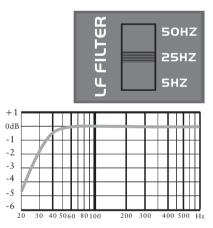
When LF cutting is at 5Hz, the audio signal can be amplified really. Like the below drawing:
