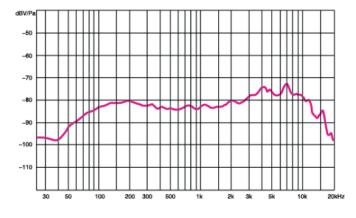
Directivity: Output connections: Frequency Response : Sensitivity: Load Impedance: Dynamic XLR (3-pin) 50Hz - 13KHz -52(+/-3dB)(0dB=1V/Pa at 1kHz) ≥600Ω±20%
