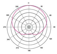
Directivity: Uni-directional Output connections: XLR (3-pin) Frequency Response: 50Hz - 16KHz
