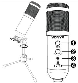
Attach the microphone holder to the tripod by turning the mounting ring counter-clockwise. Repeat to mount the microphone in the microphone holder: turn the mounting ring of the microphone holder counter-clockwise to fasten the microphone securely.
