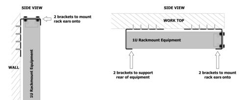
Secure the rack ears through the mounting holes as shown using the supplied screws and hex nuts provided. For 2U models, it is possible to mount a single 2U appliance or 2 x 1U appliances if required.
