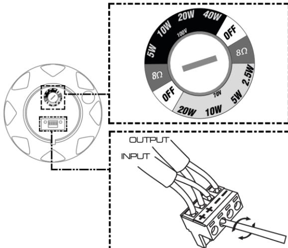
**NOTE:** Cabling of a 70/100V system may only be carried out by a qualified electrician! The total load must not exceed the rated power of the amplifier. If the 70/100V system is turned on, turn it off before connecting. Make sure the rotary switch on the speaker is turned to "off" before connecting.
