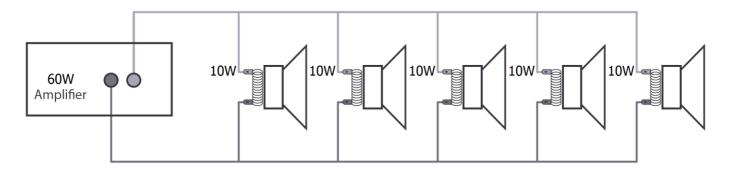
A 100V line speaker system can comprise of many speakers connected together. The determining factor for how many speakers can be used on a single amplifier is the power rating. For most purposes, it is advised to connect as many speakers as needed with a combined wattage of no more than 90% of the amplifier's output power rating.
