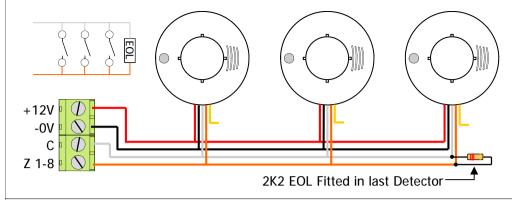
Multiple Detectors in Series Connection (using N/C Contacts) Daisy-chain wiring
