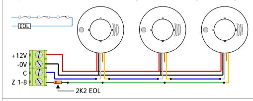
Multiple Detectors in Series Connection (using N/C Contacts) Individual wiring
