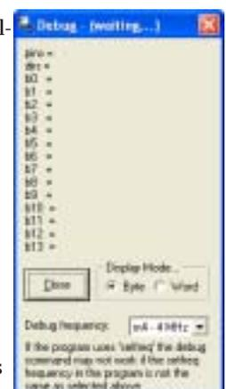
The debug window opens automatically after a download, but can also be opened manually at any time via the PICAXE>Debug menu.
