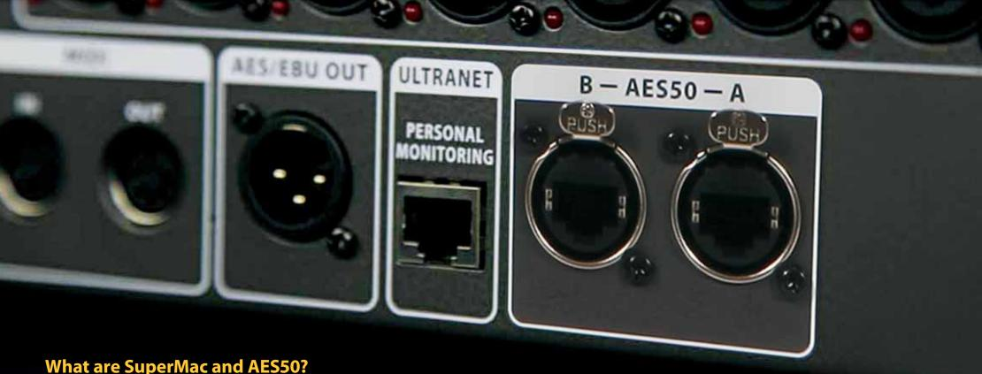
SuperMAC from KLARK TEKNIK simultaneously provides high channel counts, extremely-low deterministic latencies, accurate phase-aligned networked clock distribution, error detection, network redundancy, simple deployment and ease of use to meet the needs of the live performance industry.
