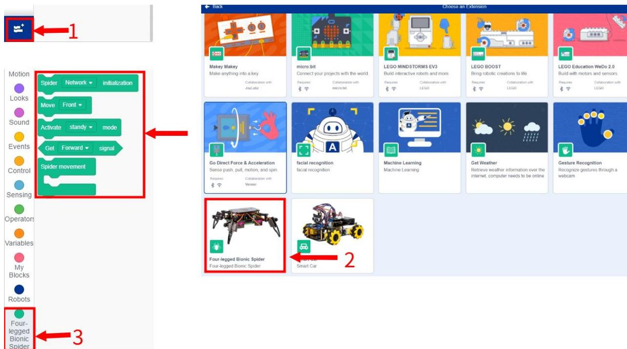
After adding the Four-legged Bionic Spider extension, you can use these two blocks to set the robot to complete a specified action or motion mode. You can also click the drop-down box in the command to select a different motion or mode.
