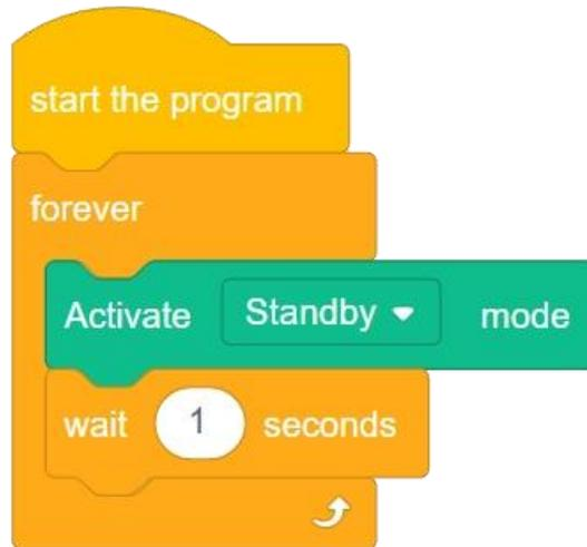
After uploading the program, we will find that the four arms of the robot are arranged in the shape of "X", and the four paws are also changed into the state of internal button to control the posture of the robot standing up. This is the standby state.
