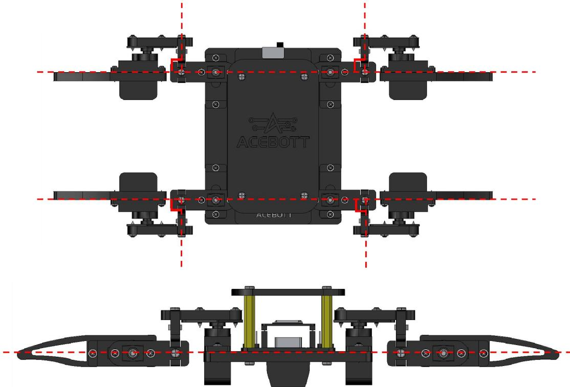
Before assembly, we have uploaded the zeroing program of the servo. During assembly, we have installed the robot as shown in the figure. This is the initial posture of the robot, that is, the zeroing position.
