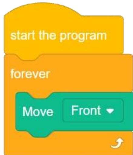
After uploading the program, it can be found that the arm paws on the diagonal side of the robot do the same action, and the two diagonal arm paws move forward in an alternate running action.
