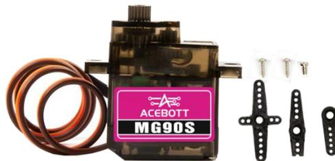
② Servo pin definition: brown line -- GND, red line -- 5V, orange line -- signal.
