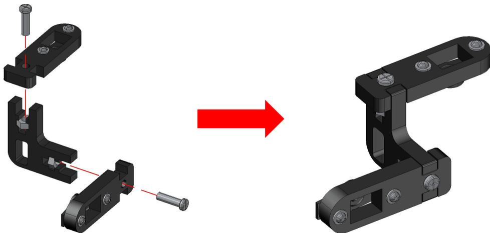
**Attention:** Similarly, install the remaining three, the effect after installation is shown below, pay attention to the direction, be sure to be consistent with the picture (2 to the left, 2 to the right).
