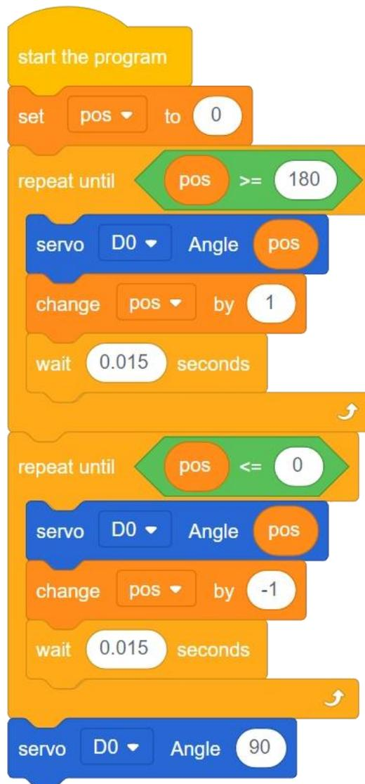
②If the steering gear is normal, it should rotate from 0 degrees to 180 degrees, then from 180 degrees to 0 degrees, and finally to 90 degrees.
