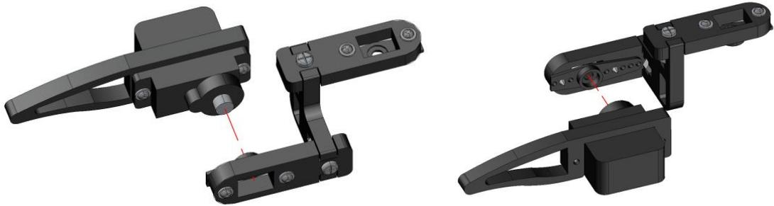
(4)Before fixing the four servos on the steering wheel, the servo line should be passed through the line hole, in addition, the steering wheel is not fixed here, and do not turn the servo during installation, as shown in the following figure.
