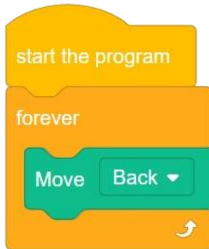
After uploading the program, it can be found that the arm paws on the diagonal side of the robot do the same action, and the two diagonal arm paws move backward in an alternate running action.
