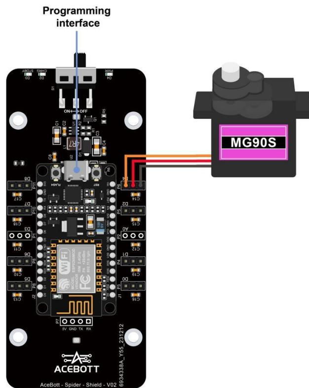
⑤ The columns with letters on the expansion board are signal pins, as shown in the following figure.
