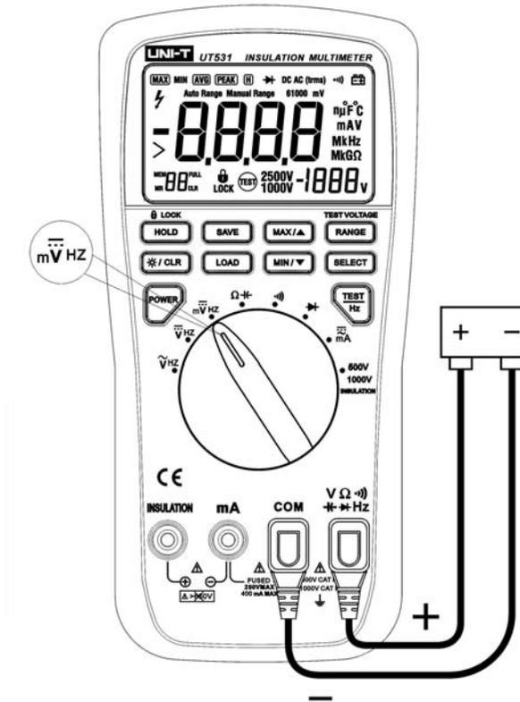
Figure 7.Measuring DC Millivolts
