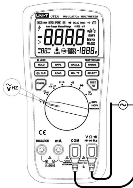
Figure 5. Measuring AC Voltage
