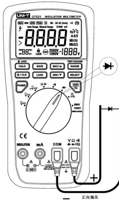
Figure 11. Testing Diodes
