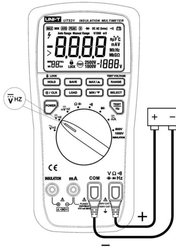
Figure 6.Measuring DC Voltage
