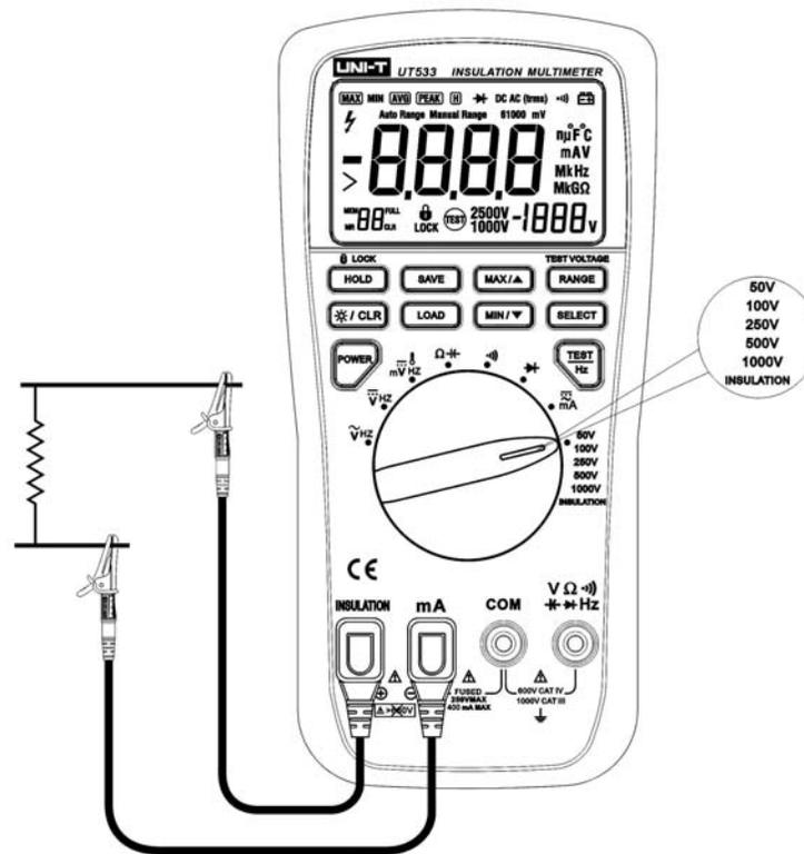
Figure 15. Testing Insulation
