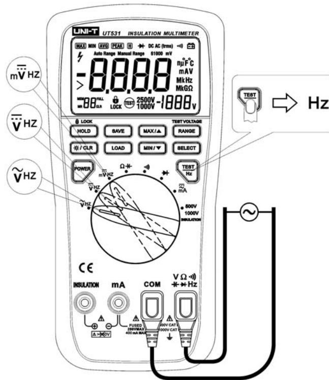
Figure 13.Measuring Frequency
