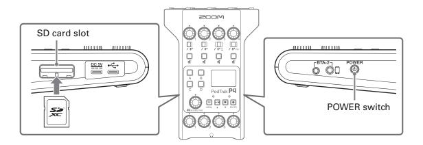
1. With the power off, open the SD card slot cover, and insert an SD card all the way into the slot.
