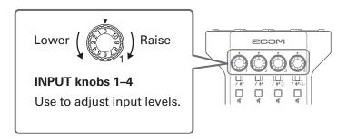
Input levels are shown on the display. While balancing the mix of the channels, adjust their levels so that they are between –12 dBFS –6 dBFS.
